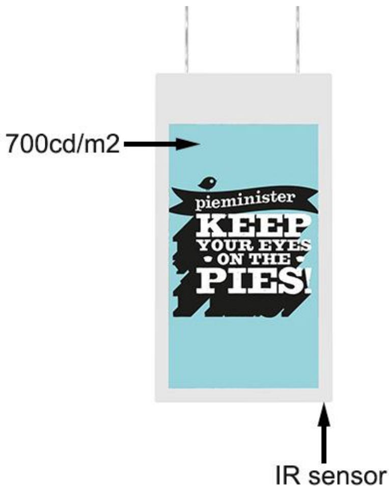
Figure 7 Location of IR Sensor from High Brightness Side
